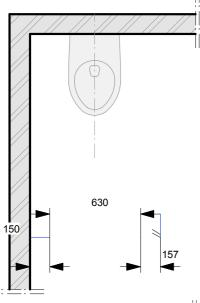
c) Then measure the last pilaster and indicate it on the floor starting from the last line. Pilaster 150 mm + 7 mm = 157 mm (this to get the outside of the corner L-profile), draw a line + 2 diagonalal stripes; this indicates the outside of the corner L- profile.
