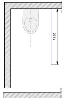
1. Measure the depth of the side division from the rear wall to the front of the cubicle, this to install the pilasters correctly and draw a line on the floor.
