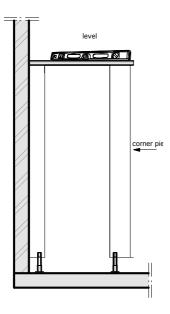
13. Now, slide the panel in the wall U-profile. Press the head rail against the wall U-profile, lift the pilaster up to the head rail and tighten the leg or jack (if there are no legs).
