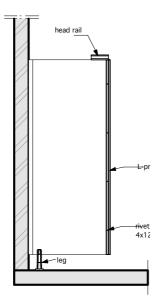
6. Now you can place the pilaster on the side division with the help of a small piece of the head rail. Press the head rail on the side division and slide the pilaster with L- profile against it, drill and rivet with Ø 4 x 12 mm. P.S. For this, you'll need assistance in the beginning.
