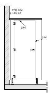
17. The door has to fit to the front pilaster both above and below, when this is the case, fix the legs (2 screws per leg) and rivet the side division at the rear wall.
