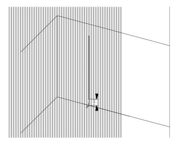
4. Now place the side division on top of 2 jacks. (1 in the front and 1 at the rear wall) You get the correct height by placing a piece of the head rail on top of the side division and adjust with the jack, in such a way the head rail just touches the wall U-profile. Then you place the level against the front side of the division and level vertically with the front jack.
