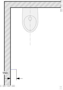
2.a) Now measure the first pilaster based on the installation drawing. Start on the left side with 150 mm and draw a line on the floor.
