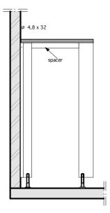
16. Fix the door and adjust the joints above and at the closing side. Adjust by pulling the small wall pilaster slightly out of the profile. When correctly positioned, rivet the wall U-profile and pilaster.
