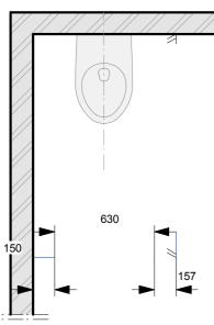
d)Transfer this last line back to the rear wall, parallel with the joints of the floor tiles (see illustration). This line is the outside of the rear wall U-profile.
