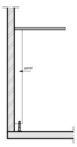
14. Now push firmly against the side wall, so the head rail fits to the wall. Hold the spacer to the pilaster on the division panel and adjust the front pilaster in the wall U-profile. Drill a hole Ø 4 on the inside and rivet.
