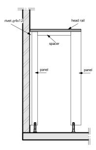
15. Then fix the head rail (see illustration). Drill 2 holes Ø 4 per pilaster and fix with screws Ø 4,8 x 32. Tighten only the first screw in the front pilaster next to the wall, in order to be able to adjust further.
